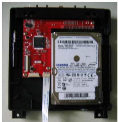
Use the supplied screws and tool to mount the Disk to the SunDriver.
